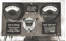
Left: When the lower plc ture was taken, Ethyl had been fed into the carbureter. The wattmeter shows that the power has risen to the maximum; the tachometer shows a corresponding in-crease in revolutions per
